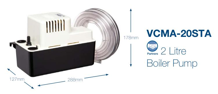
This 2 litre tank pump has one of the largest drink cycles on the market, pumping 750ml of condensate each time it is switched on. This volume helps reduce on/off cycling and can reduce the risk of external pipework freezing. In typical operation this pump only switches on for between 20 and 40 seconds and runs for around 3 to 4 hours per year. Suitable for boilers upto 200kW.
